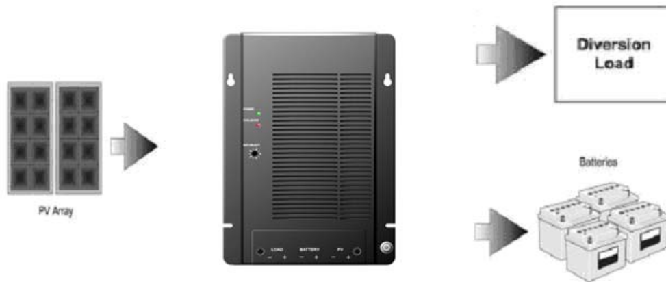
Figure 1 – 2: PV charge and load controller
